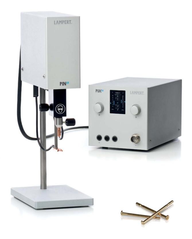
The PIN module broadens the range of the PUK® fine welding devices to include a completely new welding function. Using the PIN module, ear studs are welded onto the work piece by means of a unique electronically-controlled lifting action.
